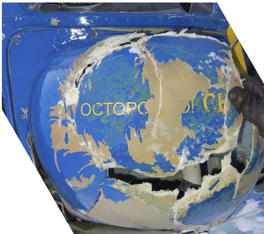
Figure 8: Parts of the radome had been torn off. The picture shows the dome after it was put back in place. Green paint from the hangar wall was deposited on the cover.
