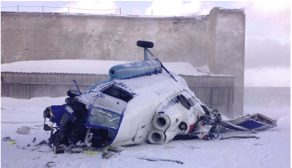
Figure 7: Picture of the helicopter taken shortly after the accident. Note the four marked impact marks from the main rotor in the hangar wall.
