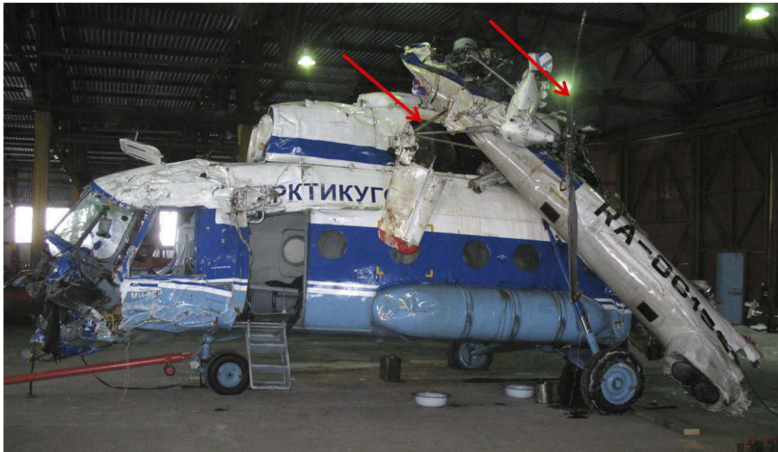
Figure 9: The damage on the left side of the helicopter. The tail rotor and the undamaged support at the rear of the tailboom are marked with red arrows.
