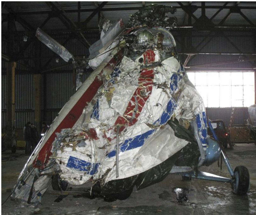
Figure 10: The damage in the transition between fuselage and tailboom. The tailboom and tail rotor on the left in the picture.
