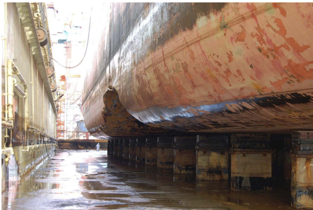
Figure 8: Damage forward of midship on the starboard side of Full City; here seen in the dry dock near Gothenburg. (Photo: AIBN).
