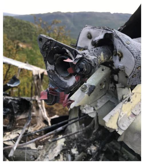
Figure 29: The broken drive shaft for the tail rotor between the fuselage and tail boom, with typical rupturing of the flexible coupling. Photo: NSIA
