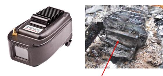
Figure 21: Appareo Vision 1000 in undamaged condition, and in severely fire-damaged condition as found in LN-OFU. The arrow points to the casing around the built-in memory module. Source: Appareo Systems, LLC and Airbus Helicopters
