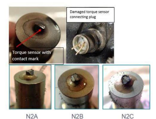
Figure 64: The torque sensor with contact mark on the pick-up part, the damaged connecting plug and the three undamaged N2 sensors. Photo: Safran Helicopter Engines/NSIA
