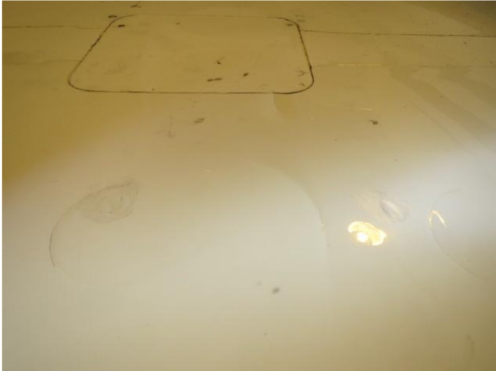
Figure 1.6 Raised Areas on RH Upper Stub Wing Skin
